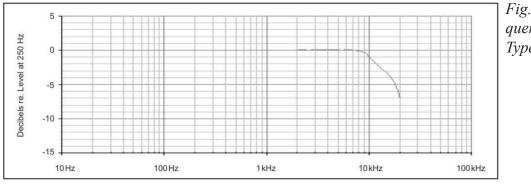
Fig. 2 Typical frequency response for Type 40EN
