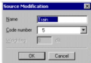
The **Weighting** field in dB corresponds to a correction factor that will be applied to all data coded with this type of noise source. It can be used, for example, to simulate how overall levels would be affected if the given noise event was reduced by N dB.
