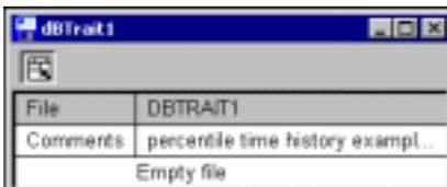
3 Create a new CMG datafile by the command **File / New** and give a name to this file. An empty datafile is created and its information window is shown on screen.
