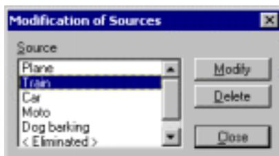
Use the command **Source / Modify** to change or remove the different types of existing sources in **dBTRAIT32**. The following dialog box is displayed on screen:
