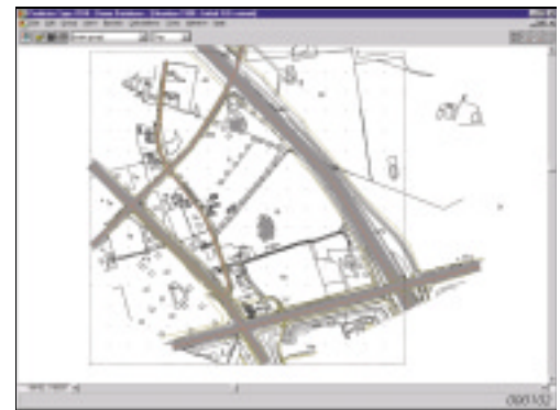
A simple model of a rural motorway with junction showing road sources, acoustically hard ground regions, topographical contours, and some receiver points at building facades
