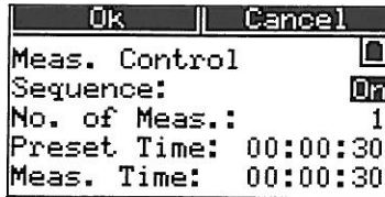
Fig.3.4 The Measurement Control Window
