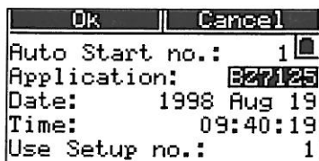
Fig. 4.3 Auto Start set-up
