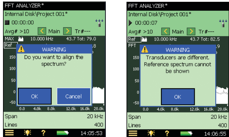
Fig. 6.3 Message boxes that appear: Left: when parameters of spectrum are different Right: when the transducers are different
