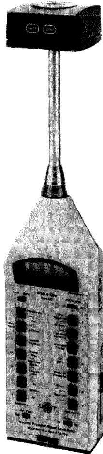
Fig.2.1 Positioning the calibrator on a Modular Precision Sound Level Meter Type 2231
