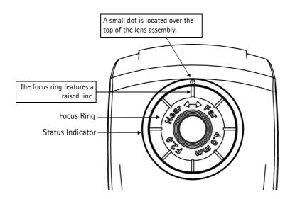
Adjust the focus ring until the raised line is aligned with the dot above the lens. The camera should now be in focus.
