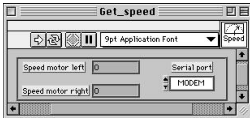
Figure 19: Get_speed panel - 2 indicators showing each wheel speed
