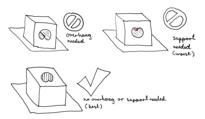
This last example illustrates how some objects are impossible to build without support in some orientation, but perfectly possible in other orientations.
