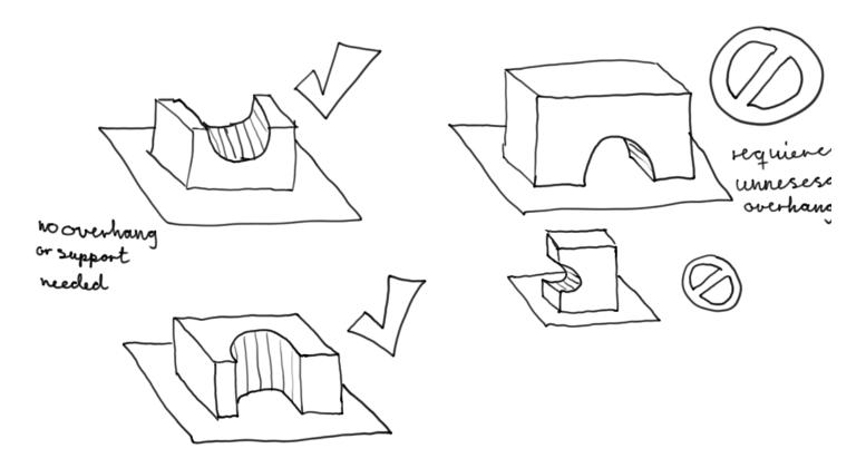
The example above shows how to orient an object to avoid the need for support.
