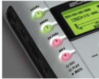
\*While in 4-track mode, the H4 records as 16-bit/44.1kHz WAV files.
