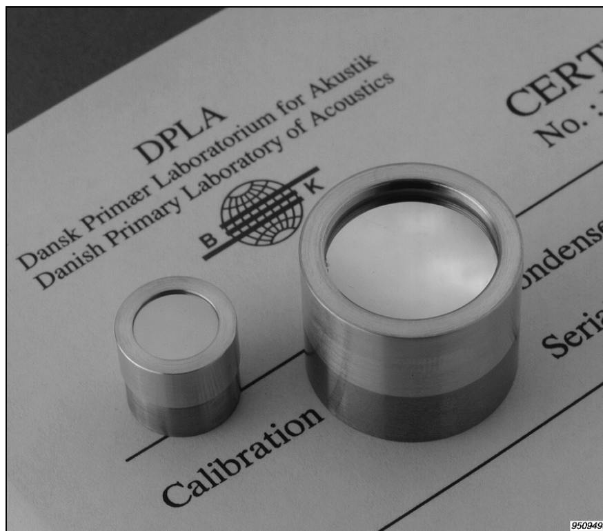
Fig.1.2 Microphone Types 4180 1/2" and 4160 1" are used by DPLA as highly stable reference microphones for laboratory calibrations
