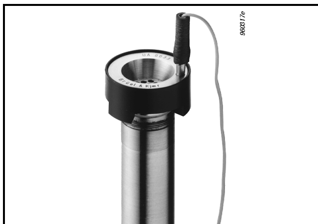
Fig.2.35 Electrostatic actuator used with a 1/2 " microphone
