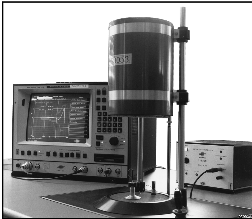
Fig. 1.9 Microphone calibration, at the end of production, using an electrostatic actuator
