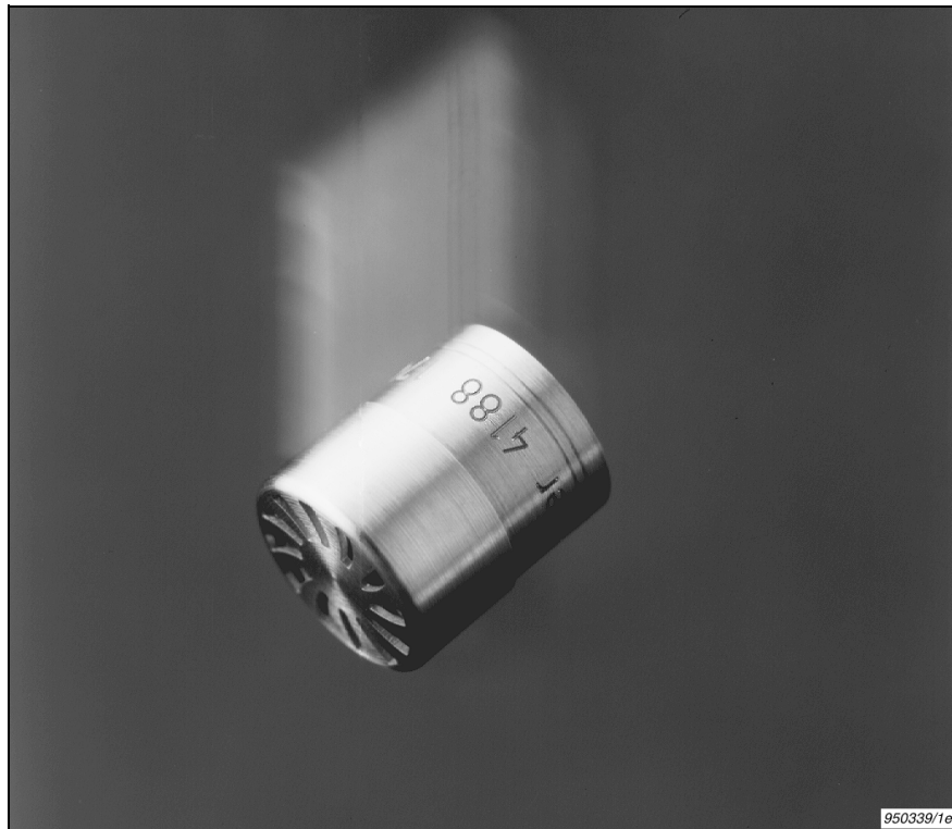
Fig 1.5 Microphone undergoing shock tests
