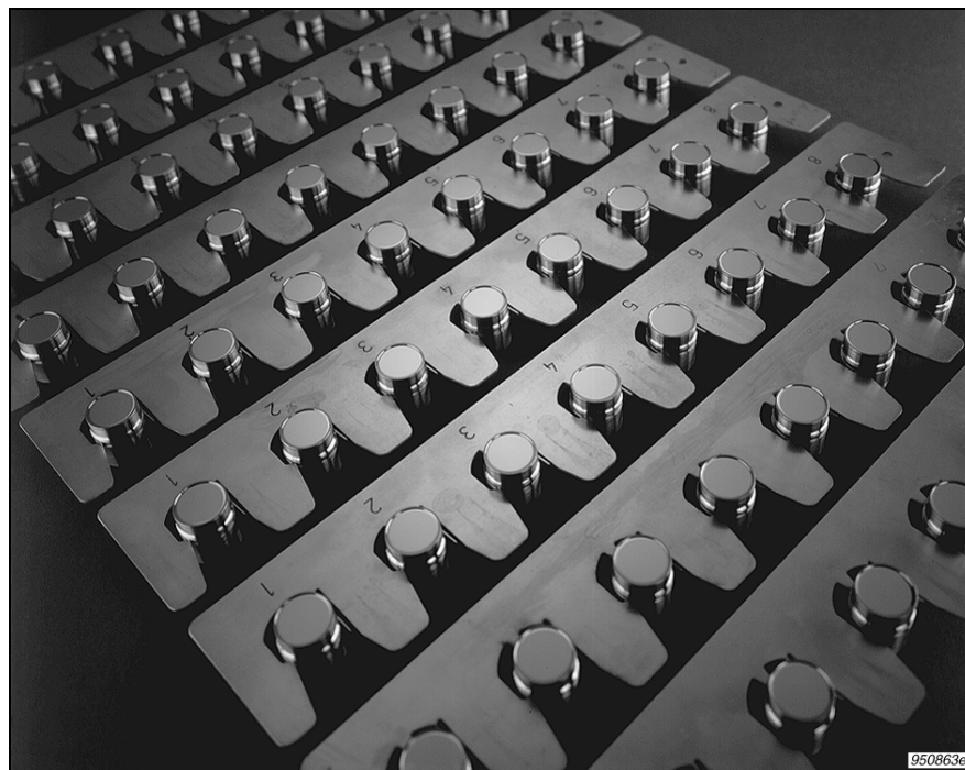
Fig. 1.7 Pre-polarized microphones nearing the end of production
