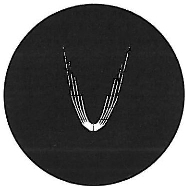
Fig. 21. Oscilloscope photograph of the B & K True RMS rectifier characteristics as used in the Electronic Voltmeter Type 2409/2416. The same quantities are traced as in Fig. 19.
