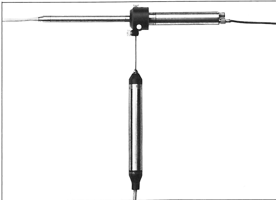
Fig. 3.7. Calibration Coupler UA 0922 with reference microphone (left), transmitter microphone (right) and probe microphone (bottom)
