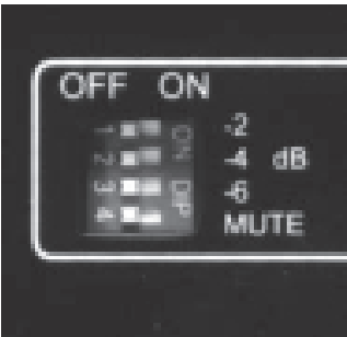
Calibrated Tilt switch. MUTE disconnects the channel for testing.
